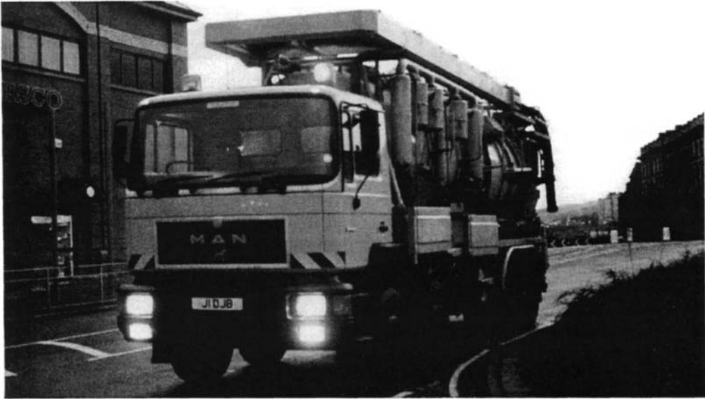
Figure 9.1 Müller combined suction/jetting machine with water recycling facilities. This machine has the following features:
