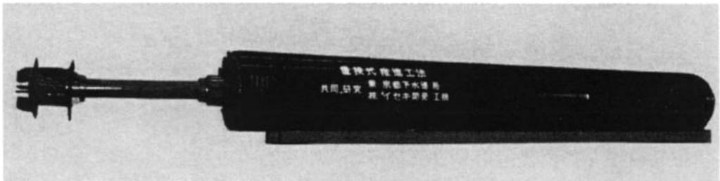
Figure 18.13 Excavator of slurry system.
