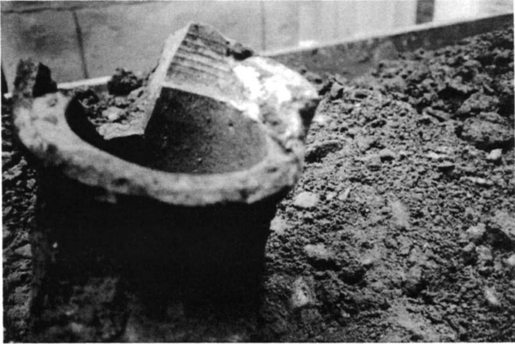
Figure 17.7(b) The offending cast-iron water main that fractured.
