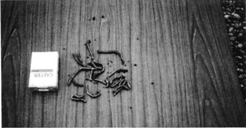
Figure 18.14 Reinforcement bar after excavation.
