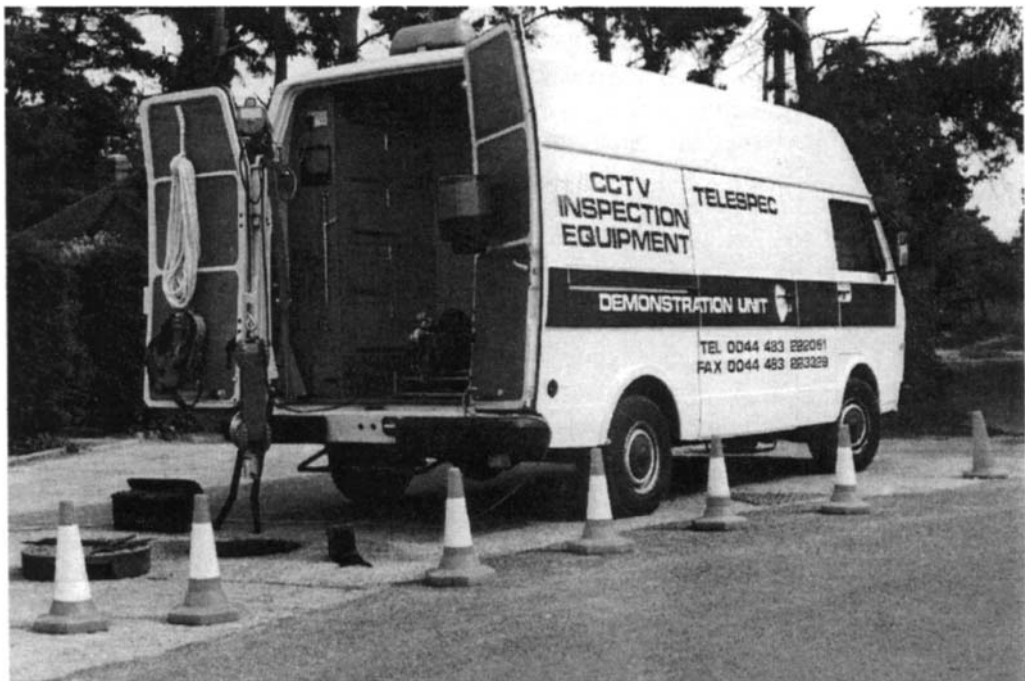
Figure 5.6 Back of survey vehicle showing camera, winch and hoist. (Courtesy of Telespec Ltd.)
